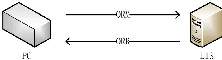
**Figure 3 Communication process of querying work order information**
